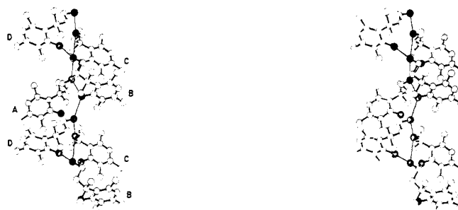
Figure 6. Stereodiamgram of diol molecules A, B, C, and D showing the continuous chain of hydrogen bonds parallel to the a axis. The c axis is horizontal.
